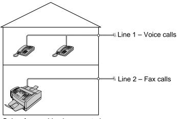
Only a fax machine is connected.
