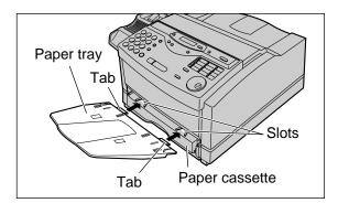
$\label{eq:2} 2 \quad \text{Open the paper tray extender by pressing $``\nabla"$} \\ \text{marked area.}$
